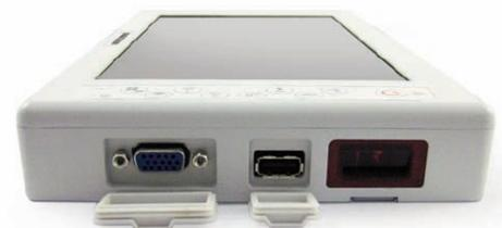
All of the MCA9's ports are on the left and the right side of the device. The optional dock adds three USB ports, a RS232 serial port, a LAN port, and DC power. The dock attaches to the bottom of the unit and also provides various mounting options.
