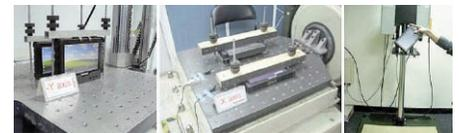
As far as sealing against the elements goes, the MCA9 carries impressive IP65 ingress protection where the "6" means the unit is totally protected against dust, and the "5" means the machine is protected against low pressure water jets from all directions, although limited ingress is permitted. The standard operating temperature range is a very wide 32 to 140 degrees Fahrenheit.
